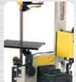
Vertical cutting position
